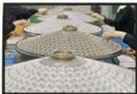
Lenses undergoing Super-Multi-Coating process.
